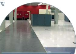
Acterna Provider of Network Soulutions Traffic lane — Integration of Vinyl on concrete access floor with Epoxy
