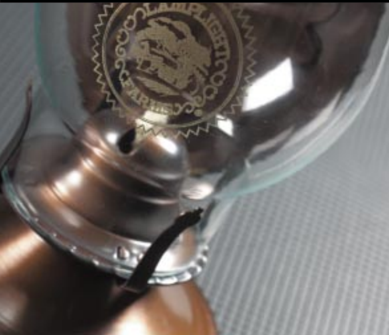
Lase curved surfaces with an optional cylindrical attachment. Color applied with powdered element. Customer logo scanned directly into Xenetech Graphic Workstation. (See page 13)
