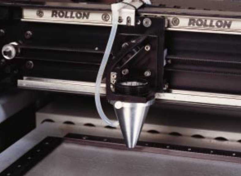
Laser engraver with air assist option
