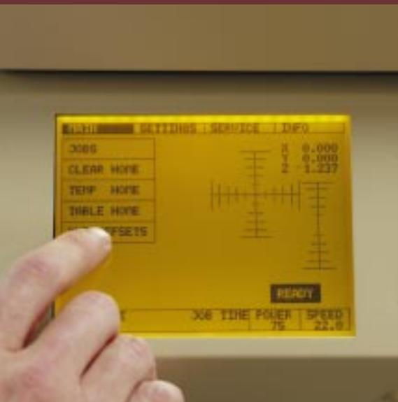
Touch screen keypad: On-board control panel gives total control of the job and view of job statistics such as, scroll-through job queue, recall job, end-of-job signal, job time statistics, positioning and more.
