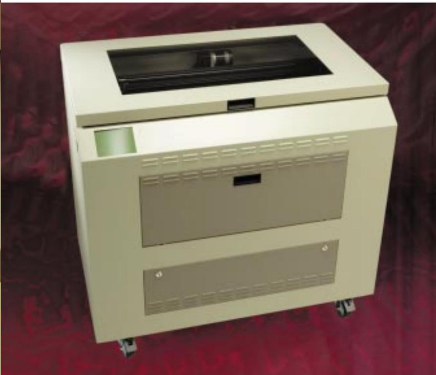
**Specifications** Table surface area: 13" x 25" (33.02 x 63.5 cm) • Engraving area: 325 sq. in. • Machine Weight: 275 lbs. (124.85 kg) • Shipping Weight: 520 lbs. (236.08 kg) • Maximum Z travel: 10" (25.4 cm) • Ships with laser accessory kit and Xenotech Graphic Workstation Professional Engraving Software: XGW -32 • Dimensions: Width 41.5" (105.41 cm), Height 38" (96.52 cm), Depth 27" (68.58 cm) (including handle and hinges) • Call for further options and specs
