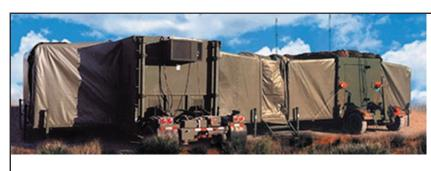
**Lightweight Mobile Shelters** are Air-, Helo-, Rail-, & Truck-transportable or detachable wheel sets can be used for transport as shown on the Tactical Operations Center complex above.
