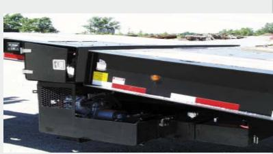
*Smooth transition from lower deck to upper deck for easier* and safer loading (Standard) Heavy duty stainless steel hinges and latch, the most durable in the industry. (Standard)
