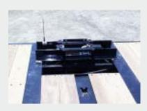
Planetary 15,000 lbs. hydraulic winch with air clutch, 100'-0" 1/2" cable w/ roller guide; tensioners & dual function wireless remote control for winch (Standard)
