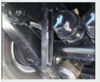
Suspension straps are mounted on the shocks to prevent over extension of the suspension air ride (Standard)
