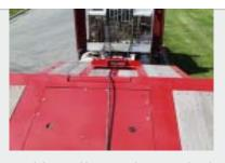
Cable roller in lower deck section for efficient loading with the winch (Standard)
