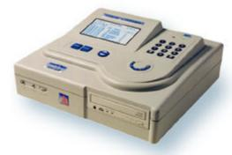
Total Recall is a compact multi-channel logging recorder with built-in display and simple navigation keys. You can listen to monitored conversations live or replay them from the internal hard drive that holds 1600 hours of conversations. Archive all or selected conversations to inexpensive compact disks with the touch of a few simple buttons — up to 180 hours on a standard recordable CD that costs less than one dollar.
