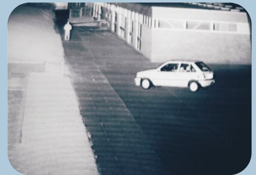
Above: In the monitor photo of a dark night-time scene, the vehicle at 150 feet (50 m), the person at 300 feet (100 m) and the fence at 500 feet (160 m) are all clearly visible because of the even-illumination provided by dual 830 nm UF500 infrared lamps.
