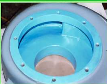
Pump housing reconditioned and machined back to OEM standards
