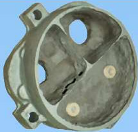
End cover with erosion holes through base metal
