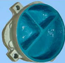
End cover reconditioned by using the 3 coat process, base, reinforcement, and top coat
