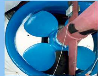
Kort and propeller coated to increase performance and eliminate cavitation & corrosion
