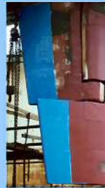
Coating of freighter's rudder tips to reduce drag and eliminate cavitation & corrosion
