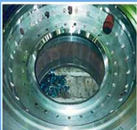
This Cylinder Cover shows pre-machining through the cooling bores, injectors, air and safety bores in prepare for welding
