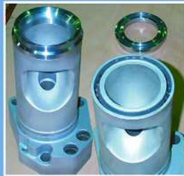
Water-cooled Exhaust Cages involve removal of seat, manufacture of new seat and welding in-place with final machining and pressure-testing
