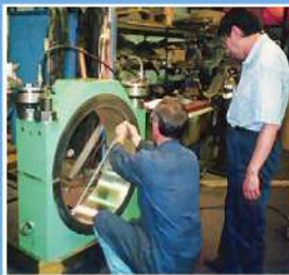
Babbitt Bearings are centrifugally cast and final machined under torqued condition to minimize fitting operations upon installation
