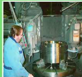
Upon completion of chroming operations, we complete the process with our grinding procedure to ensure flat and parallel ring-groove lands
