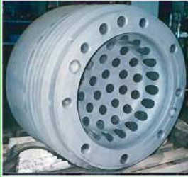
All components are sandblasted to remove any carbon deposits to aid in efficient heat transfer
