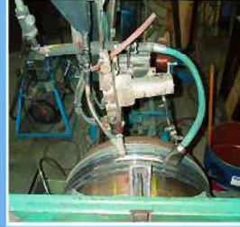
Weld build-up is performed using the latest state-of-the-art equipment and technology
