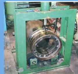
Piston Skirt rubbing band being hydraulically rolled into place before finish machining
