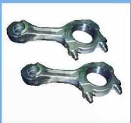
Auxiliary Conrods are cleaned, crack-detected, serrations lapped, torqued and finish ground to remove ovality
