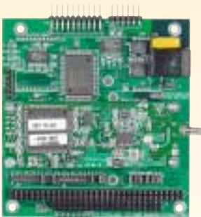
Model PXMM-GPS-XT with GPS receiver installed.
