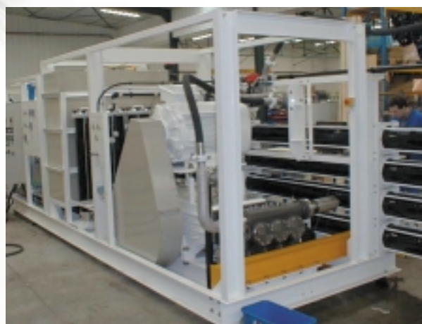
150 Frame Salt Water Reverse Osmosis Systems
