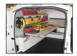
This unit can be delivered fully equipped for service operations with extras comforts such as a thermostat controlled interior for onboard climate control of A/C and/or Heat. Auxiliary 115v A/C & 12v power is available onboard through a choice of power sources. Ventilation and added insulation for extreme weather conditions is also available.
