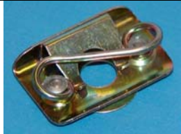
Slip-On Sizes 4 & 5 Slips over support edge and snaps into round hole.
