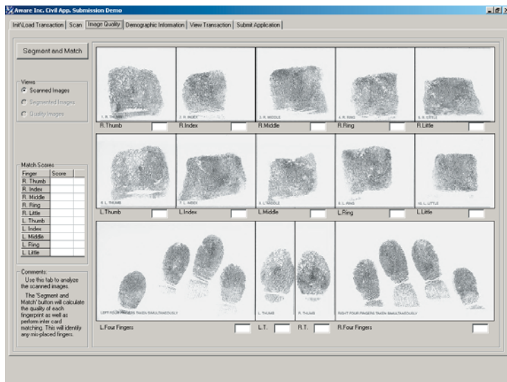
EXAMPLE LIVESCAN USER INTERFACE THAT SHOWS THE ELECTRONICALLY ACQUIRED FINGERPRINT IMAGES AND BUTTONS TO APPLY THE AWARE IMAGE QUALITY AND SEQUENCE CHECK FUNCTIONS.
