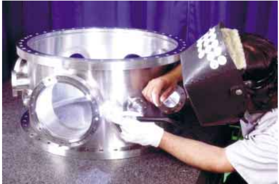
GTAW Fusion Welding
