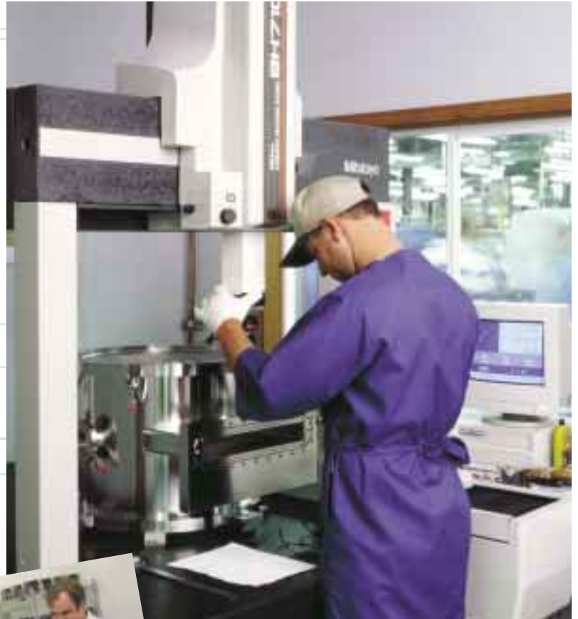
Mechanical inspection of process chamber with Coordinate Measuring Machine (CMM)
