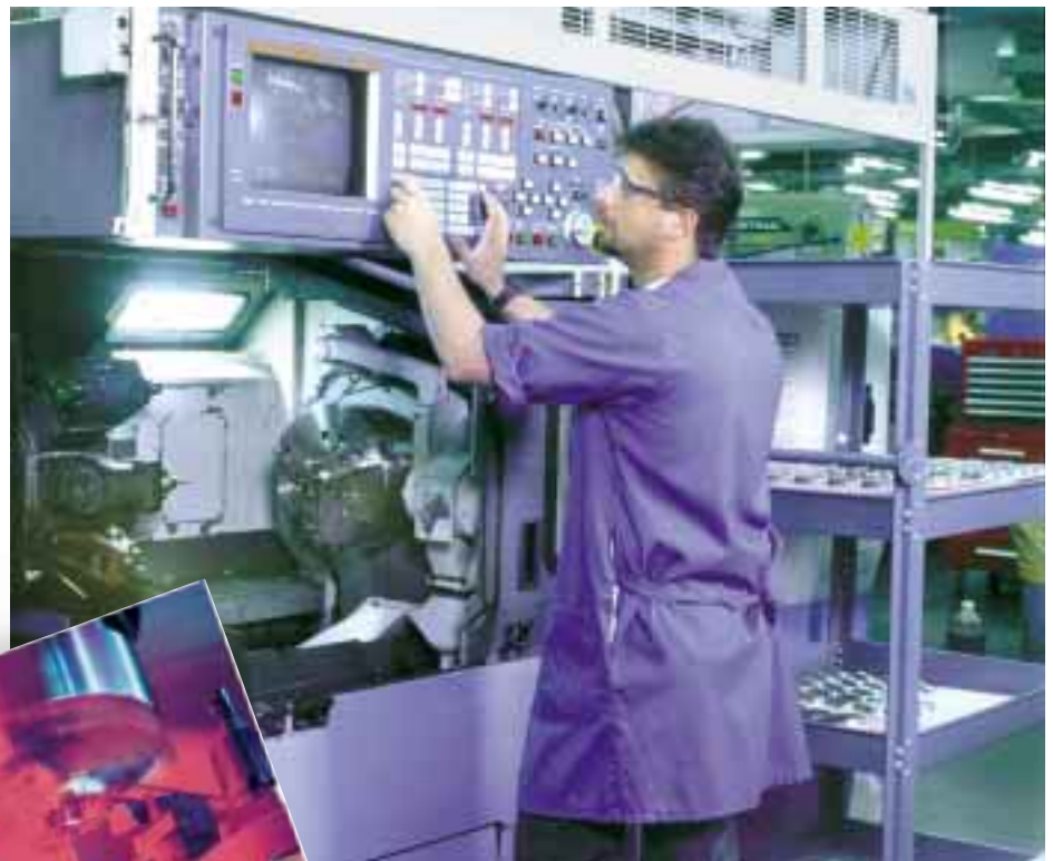
CNC Machining Center with dual spindles, live tooling and robotic gantry
