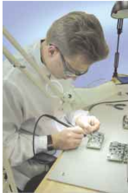
Soldering Printed Circuit Boards (PCBs)
