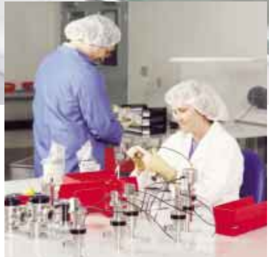
Valve assembly in Class 1000 clean room
