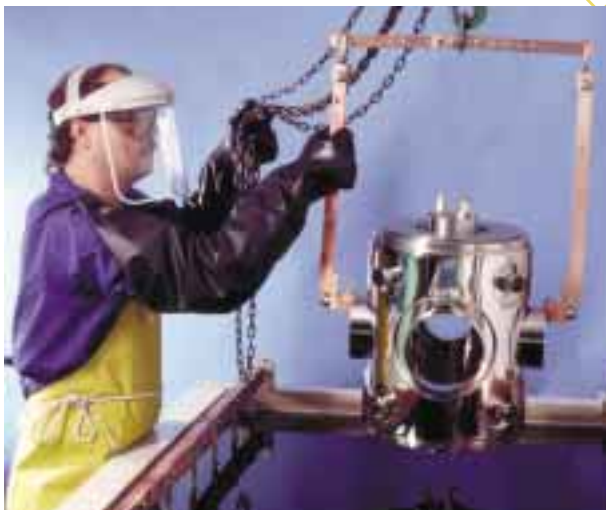
Electropolishing vacuum chamber
