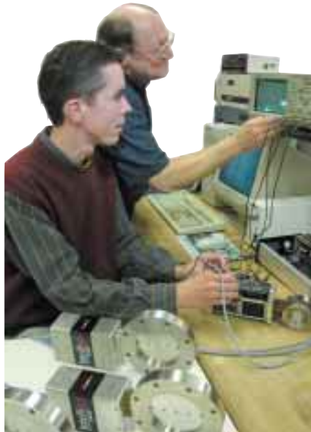
Checking wave forms on IQ Series Intellisys Throttling Valves
