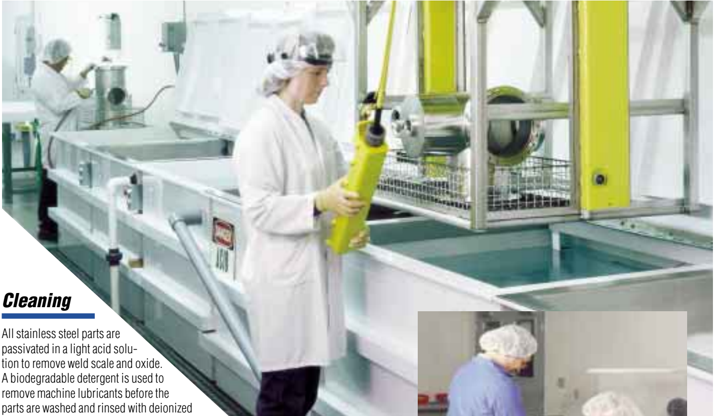
Chem cleaning vacuum chambers
