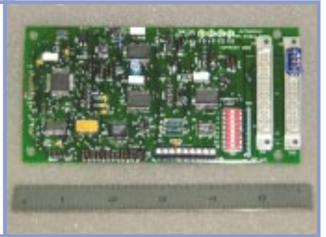
APC single-phase SCR firing module with open feature slots. DC power supply and heat sink not shown.
