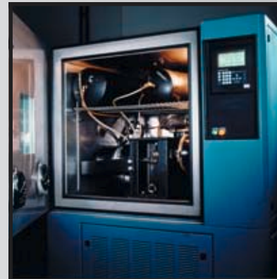
Environmental Chamber tests brakes at various temperatures.
