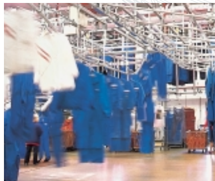
METRICON garment handling system with track and trace.
