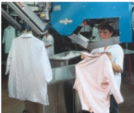
METRICON loading station. Scanning of JENTAG (laundry chip) and loading of garments.
